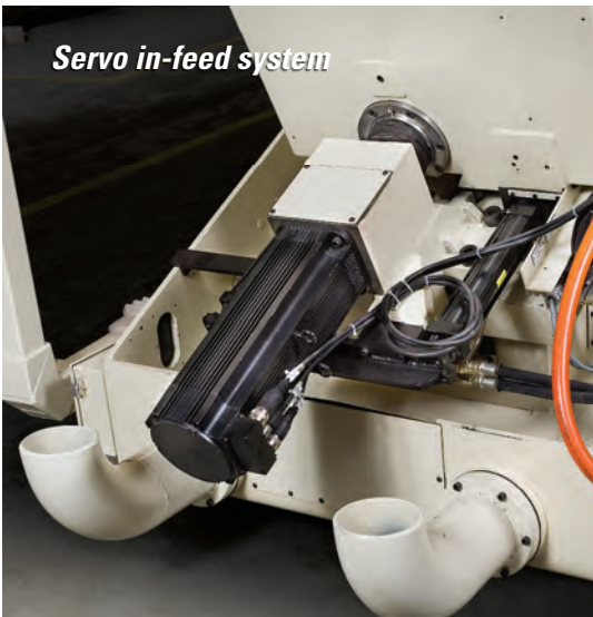
Dresser, servo and ball screw conversion
