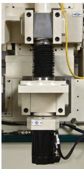
GCH servo rock feed system delivers position accuracy of 0.001mm (patent pending)
