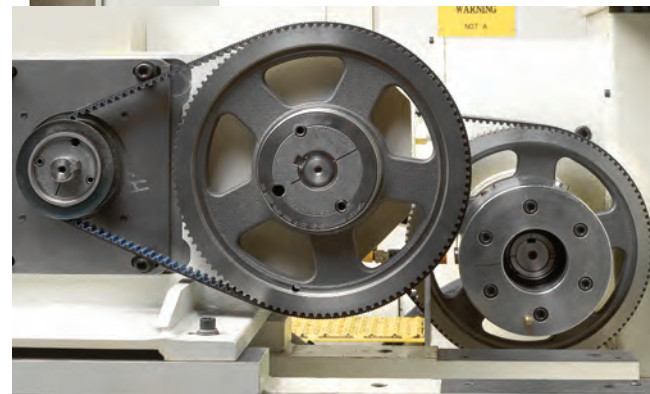
Mechanical crash protector disengaging clutch
