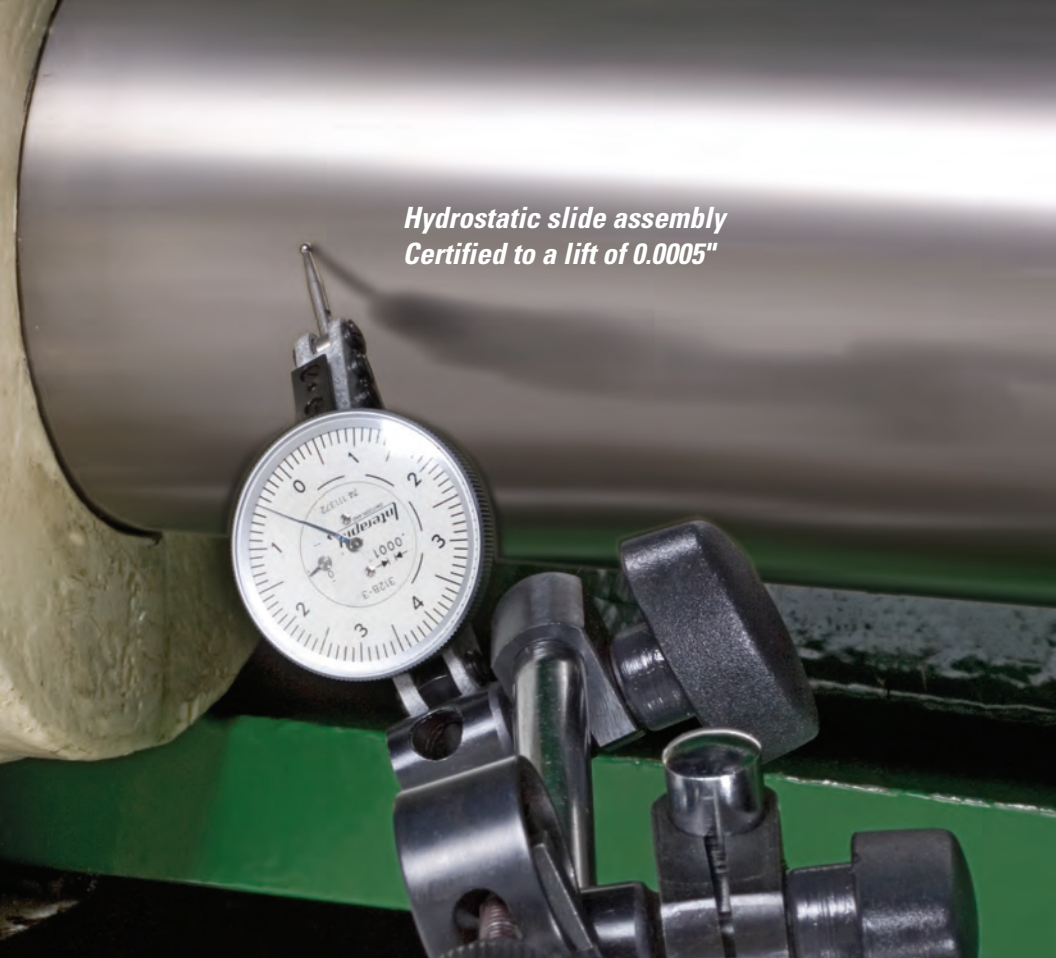
Precision regulating wheel head spindle test stand guarantees quality workmanship
